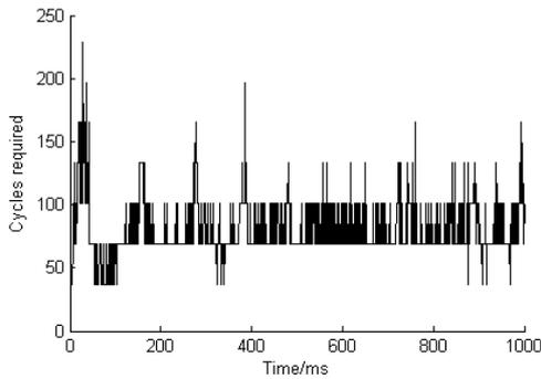
Fig. 8. Graph showing the number of cycles required per timestep for the SNN simulation of Figure 7.
