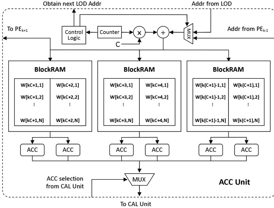
Fig. 3. Simplified architecture of ACC Unit, each Block RAM storing 2 weight tables (register and control logic omitted)
