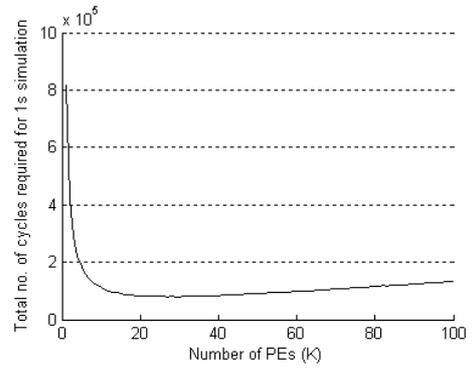
Fig. 6. Graph showing cycles per timestep as a function of  $K$ , the number of PEs used.
