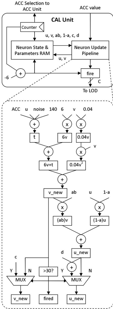
Fig. 4. Datapath of the CAL Unit (pipeline stages not shown).
