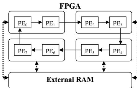
Fig. 5. A 8-PE Network using 4 FPGAs
