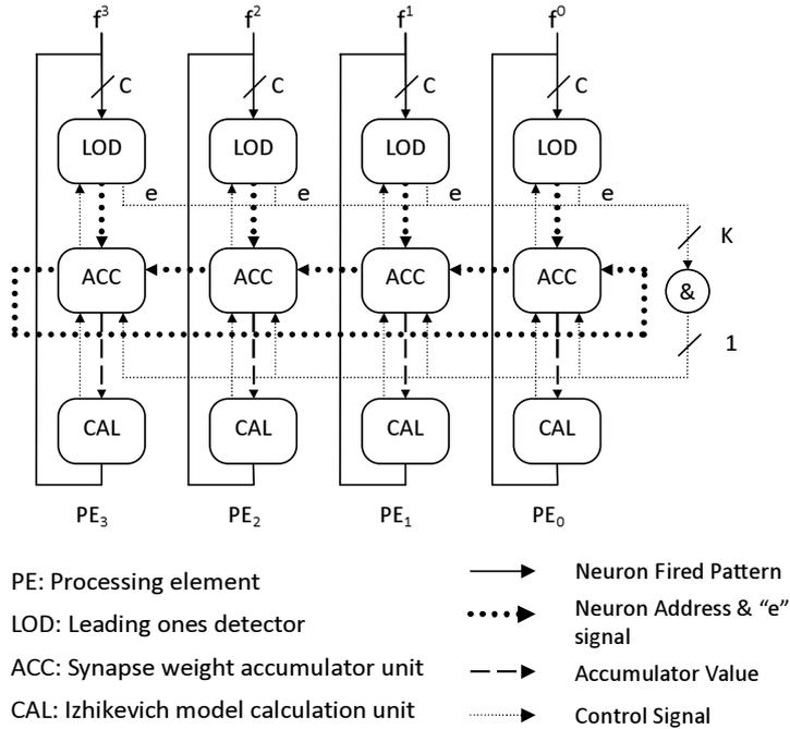
Fig. 1. Datapath of the spiking neural network simulator. Four PEs  $K = 4$  are shown, each handling  $C$  neurons. Thus a total of  $4C$  neurons can be simulated.
