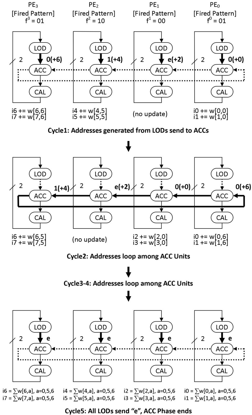
Fig. 2. ACC computation for an 8-neuron simulation. Neurons 0, 5 and 6 have fired and  $I_i$  values are accumulated in the 4 PEs, each one handling two neurons.
